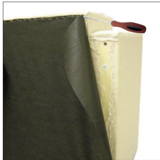
B. Using a flat head screwdriver pry out staples and remove the black lining to reveal chair framework
