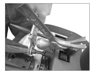
Using a curved jaw locking plier, lock the plier around the neck of the paddle.
