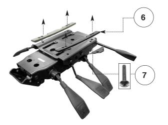
To detach the Mechanism (5) and Plastic spacers (6) From the Seat (8), unscrew the four screws (7)
