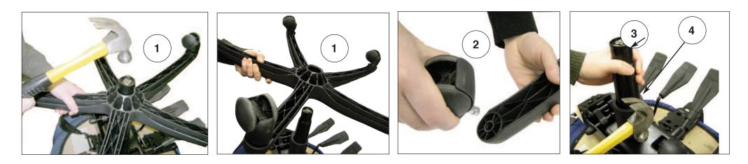
Remove the base (1) by striking the bottom edge of the Gas lift with a hammer. Pull out the casters (2) by hand. Remove the metal stem of the casters using a plier.
