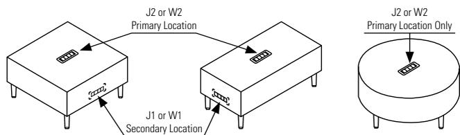
Primary location is on the top rear/edge of the unit J4 (black) or W4 (white). Secondary Location is the back side of the unit J6 (black) or W6 (white).
