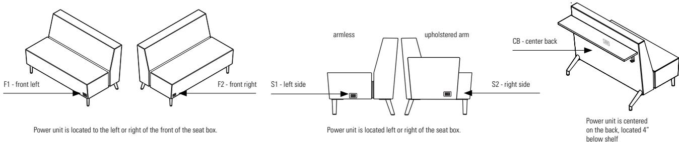
Power unit is located to the left or right of the front of the seat box.
