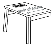
On surface power module on narrow tables
