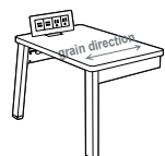
On surface power module on narrow tables
