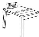
On surface power module on narrow tables
