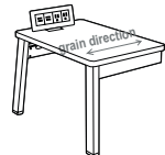
On surface power module on narrow tables
