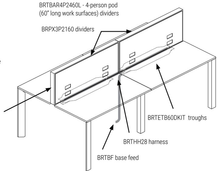
**BRPX3P dividers with built-in 8-wire, 4-circuit power distribution system and data.**
