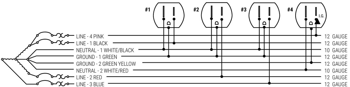
An 8-wire, 4-circuits, 3+1 electrical systems complies with UL 1286
