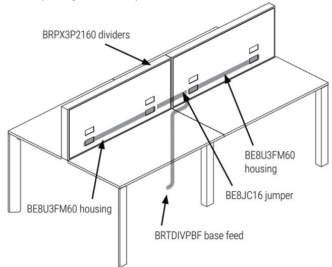
BRTBAR4P2460L - 4-person pod 60" long work surfaces dividers power troughs
