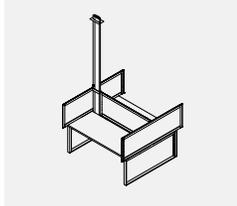
• Ceiling pole brings ceiling feed conduit and data cables from the ceiling to Power Troughs at desk height.
