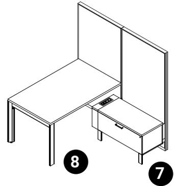
NOTE: Specify BRTHH58 (9) to distribute power from double sided, Back 2 Back below worksurface power trough to a single sided, below work surface power trough at the end of a table run.
