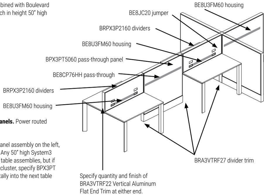
**BRPX3P dividers combined with BOULEVARD System3 panels.** Power routed through System 3 panels.
