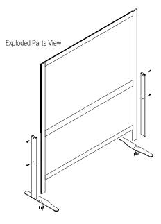
STEP 3: Align holes in the base with extruded screw ports.
