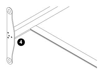
STEP 5: Insert the rear bracket into the divider's short vertical extrusion.
