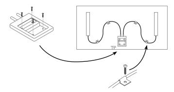
9. Secure the cables to underside of the top with the provided brackets (4).
