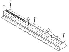
8. Position cable release mechanism in the center of the table 1" from the user edge and screw into the underside of the top.
