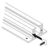
2. Use the guide to position the bolt with washer and nut 1 7/8" from the end. Tighten nut in place.
