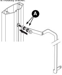
6. Attach modesty panel. Using guide block position panel 1 7/8" below support beam and screw in place.
