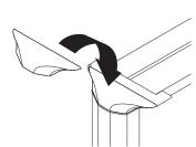
3. Snap support block into channel
