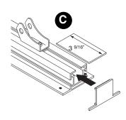
6. Connect the base to the support beam. Insure that black nylon washers (A) are installed between the pivot bracket and the assembly.
