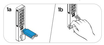
**Unlock**: Insert an assigned User Key, then turn the knob to the unlocked position. Open the door†.
