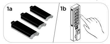
Collect all remaining and replacement Manager Keys. Go to any lock operated by lost/stolen Manager Keys. Press 5 5 5 0 -- .
