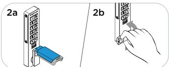
**Unlock**: Insert the same User Key then turn the knob to the unlocked position. Open the door.
