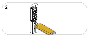
While the LED is flashing, insert the Programming Key. A two-tone beep will be heard and the LED will turn off.
