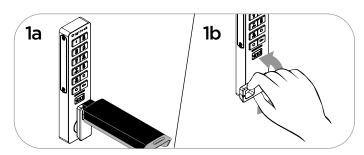
**Unlock**: Insert a valid Manager Key then turn the knob to the unlocked position. Open the door<sup>†</sup>.
