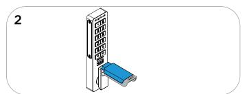
While the LED is flashing, insert a User Key. Two sets of two-tone beeps will be heard and the LED will turn off.
