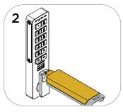
While the LED is solid, insert the Programming Key. A two-tone beep will be heard and the LED will turn off.
