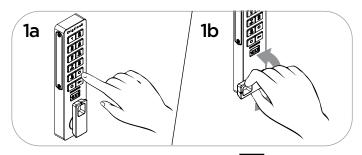
Unlock: Press [ [assigned 4-7 digit code] , then turn the knob to the unlocked position. Open the door\*†.
