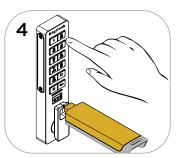
End Express Registration mode:\* Go to any programmed lock. Press C then insert the Programming Key.
