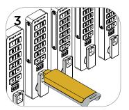
Insert the Programming Key to program each lock to operate with the same user credentials and Manager Keys. Two sets of two-tone beeps will be heard and the LED will flash twice to indicate successful programming.
