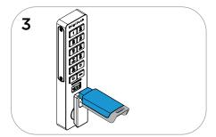
While the LED is flashing, insert a new User Key.
