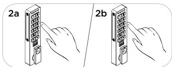
While the LED is flashing, press C [new 4-7 digit code] O-A two-tone beep will be heard.
