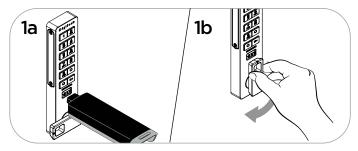
**Lock**: Close the door. Insert a valid Manager Key then turn the knob to the locked position.
