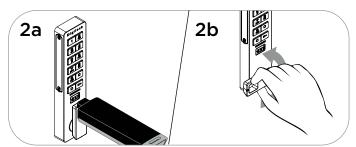
**Unlock**: Insert a valid Manager Key then turn the knob to the unlocked position. Open the door\*\*.
