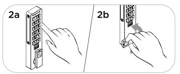
Unlock: Press [same 4-7 digit code] Then turn the knob to the unlocked position.
