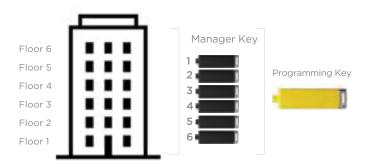
Each lock must be set up to operate with a Programming Key and Manager Key(s). See <a href="Programming First Locks">Programming First Locks</a> to program new Manager Keys to a first lock. See <a href="Express Register Manager Keys">Express Register Manager Keys</a> to register the new Manager Keys to other locks.
