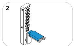
While the LED is flashing, insert the assigned User Key. A two-tone beep will be heard.
