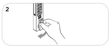
**Relock**: Close the door, then turn the knob to the locked position.
