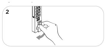
Relock: Close the door, then turn the knob to the locked position.
