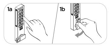
Lock: Close the door. Press [ [any 4-7 digit code] — then turn the knob to the locked position.
