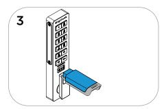
While the LED is flashing, insert a new User Key.
