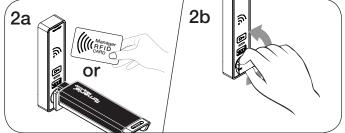
To unlock: Insert a registered Manager Key or touch on, present a valid Manager RFID then turn the handle to the unlocked position. Open the door.\*
