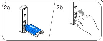
To unlock: Insert the same User Key then turn the knob to the unlocked position. Open the door.
