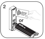
While the LED is flashing, insert a valid Manager Key or present a valid Manager RFID.
