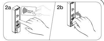
To unlock: Touch 🗹 and present the same User RFID Credential, then turn the knob to the unlocked position. Open the door.
