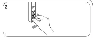
To lock: Close the door then turn the knob to the locked position.
