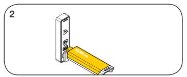
While the LED is flashing, insert the Programming Key.
