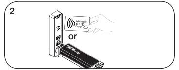
While the LED is on, insert one Manager Key or present one RFID Credential at a time.
