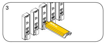
Insert the Programming Key to program each lock to operate with the same Manager Credentials.
