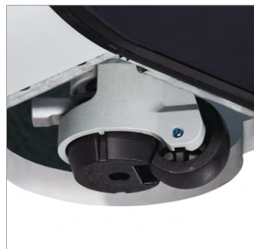
Special casters allow the acoustic pod to be easily positioned (once in place, the caster retracts allowing the leveling glide to keep the pod in its proper position)
